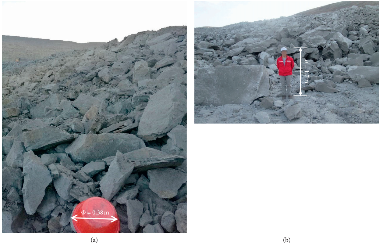
FIGURE 16: Comparative analysis of rock mass crushing. (a) Crushing result of rock mass in the test group. (b) Crushing result of rock mass in the control group.
