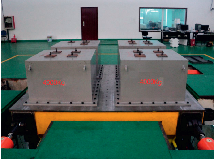
FIGURE 1: Multiaxis hydraulic servo shaking table experimental setup.
