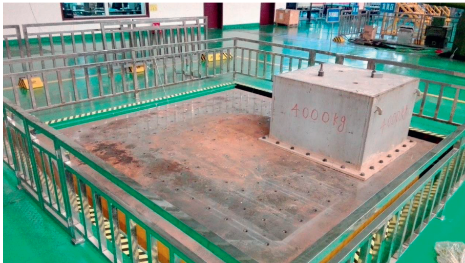
FIGURE 8: Multiaxis hydraulic servo shaking table with eccentric load.
