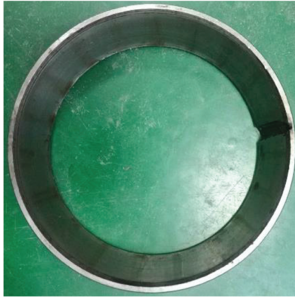
FIGURE 8: The crack fault of bearing outer ring.
