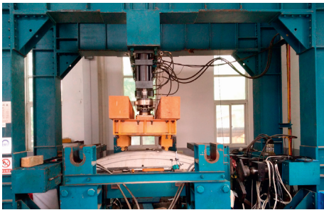
FIGURE 2: Loading system of the full-scale experiment.
