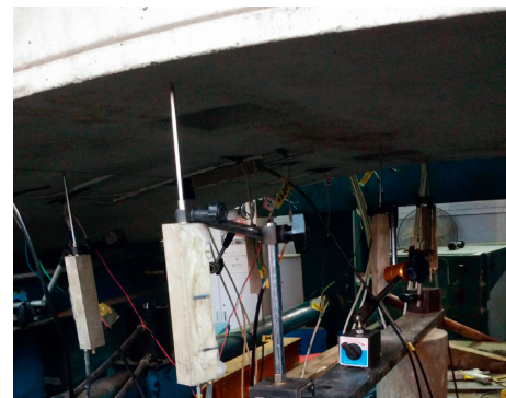
FIGURE 7: Measuring vertical displacement of the segment with displacement meter.
