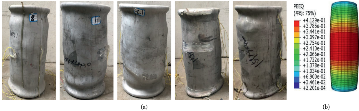
FIGURE 4: Failure mode of the specimen. (a) Experimental result and (b) FE result.
