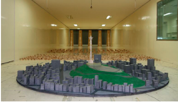
FIGURE 11: Full aeroelastic model test of the Busan tower (1 : 200 scale).
