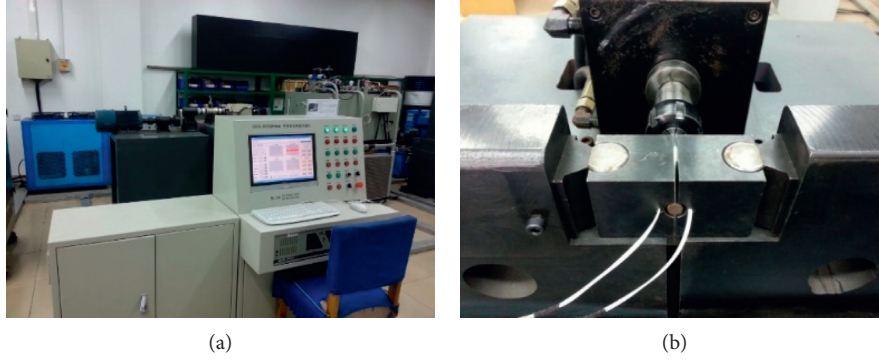
FIGURE 2: Testing machine and self-lubricating fabric liner under test. (a) Testing machine. (b) Self-lubricating fabric liner under test.
