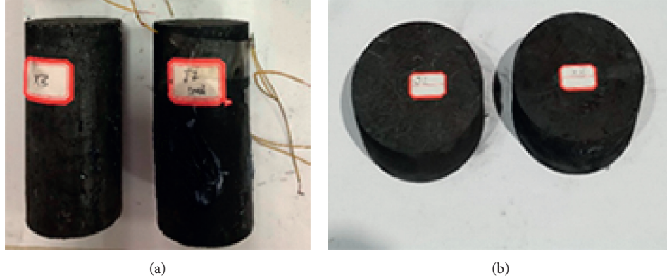
FIGURE 1: Photos of coal cores used in the experiments. (a) Cores used in the test of static mechanical properties and (b) cores used in the test of dynamic mechanical properties.
