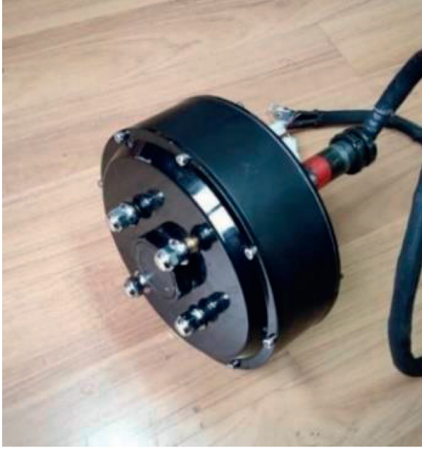
FIGURE 1: The outer-rotor PMBLDC motor.
