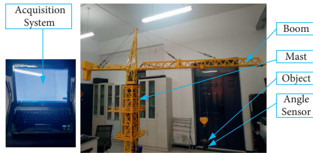
FIGURE 4: Components of the test bench.
