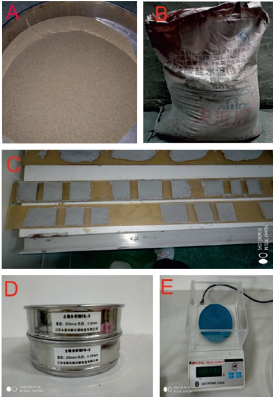
FIGURE 2: Materials and instruments used in the test: (a) Fujian standard sand for testing; (b) cement; (c) plexiglass sample after applying cement mortar; (d) soil analysis sieves with the apertures of 0.25 mm and 0.5 mm; (e) electronic scale.
