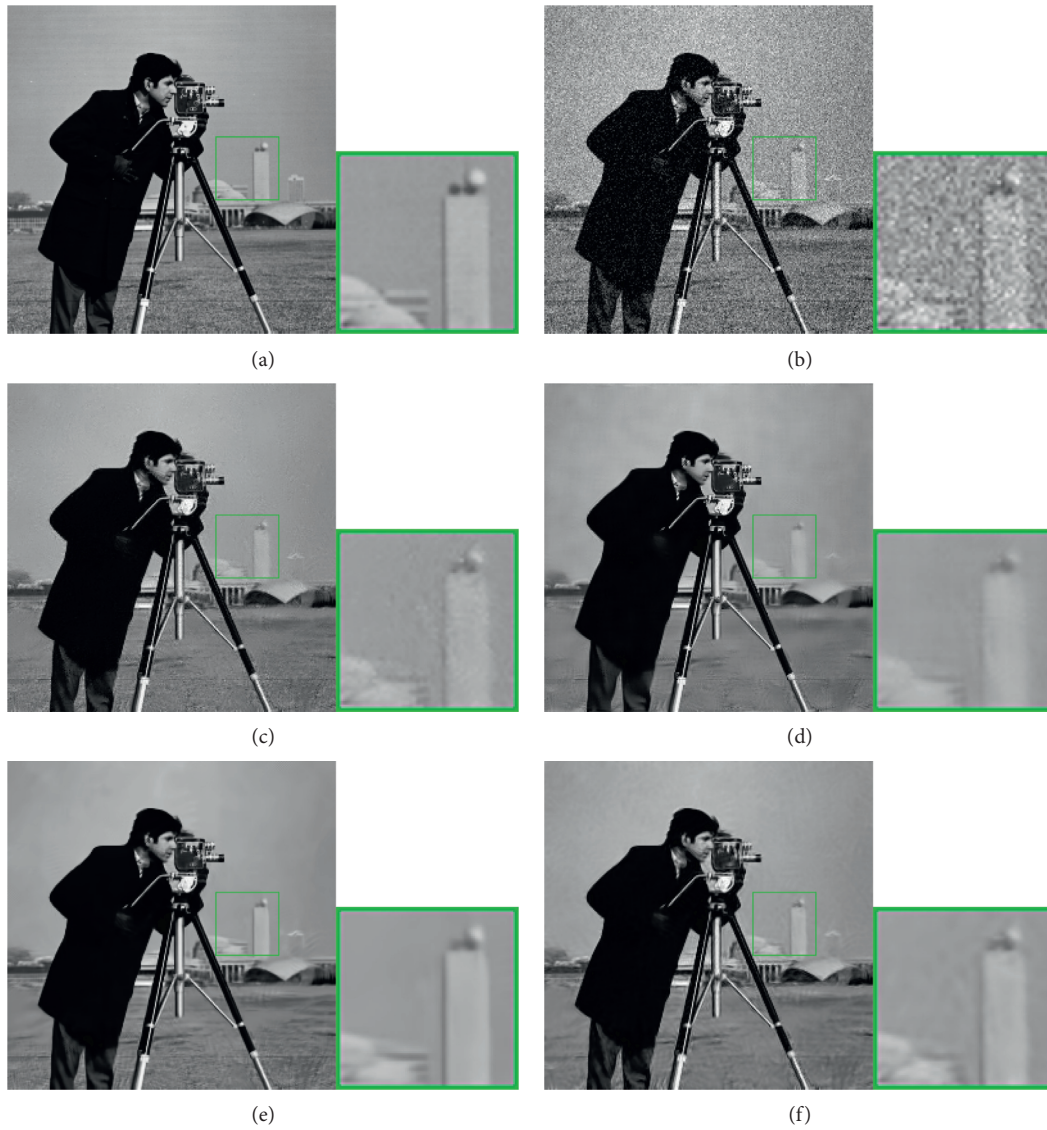
FIGURE 5: Denoising performance on the C. man image with moderate noise corruption. (a) Original image; (b) noisy image ( \sigma=20 ); denoised image (c) by NLM [21]; (d) NLM-SAP [29]; (e) BM3D-SAPCA [41]; (f) our proposed method.
