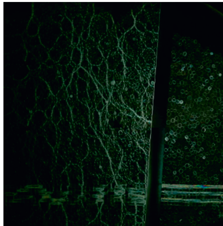
FIGURE 7: Force chains after the first excavation.
