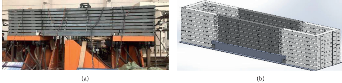
FIGURE 1: Design of the test model box. (a) Site layout of the model box. (b) Design of the model box.
