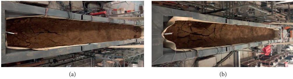
FIGURE 4: Final failure state of soil. (a) Left side. (b) Right side.
