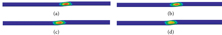
FIGURE 7: Plastic zone of lining under strike-slip fault with different dip angles. Cloud diagram of the plastic zone of the strike-slip fault with (a) 45° dip angle, (b) 60° dip angle, (c) 75° dip angle, and (d) 90° dip angle.
