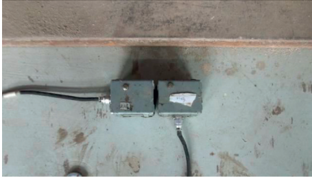
FIGURE 6: Accelerometers installed on the shaking table.
