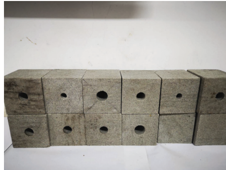
FIGURE 3: Actual pretreatment of rock samples.
