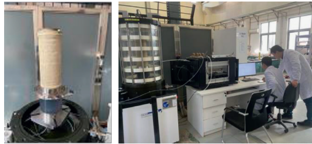
FIGURE 4: GDS large scale cyclic triaxial test of coarse-grained filling.
