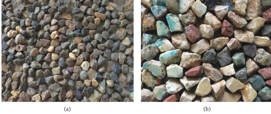
FIGURE 3: Gravel bed arrangement for (a) k_s = 1.25 cm and (b) k_s = 2.2 cm.
