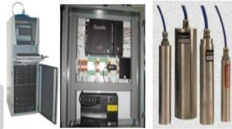
FIGURE 2: Mainframe processing system, substations, and sensors of the microseismic monitoring system.
