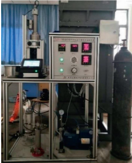
FIGURE 3: RLSS-2 seepage test device for coal rock rheological disturbance effect.
