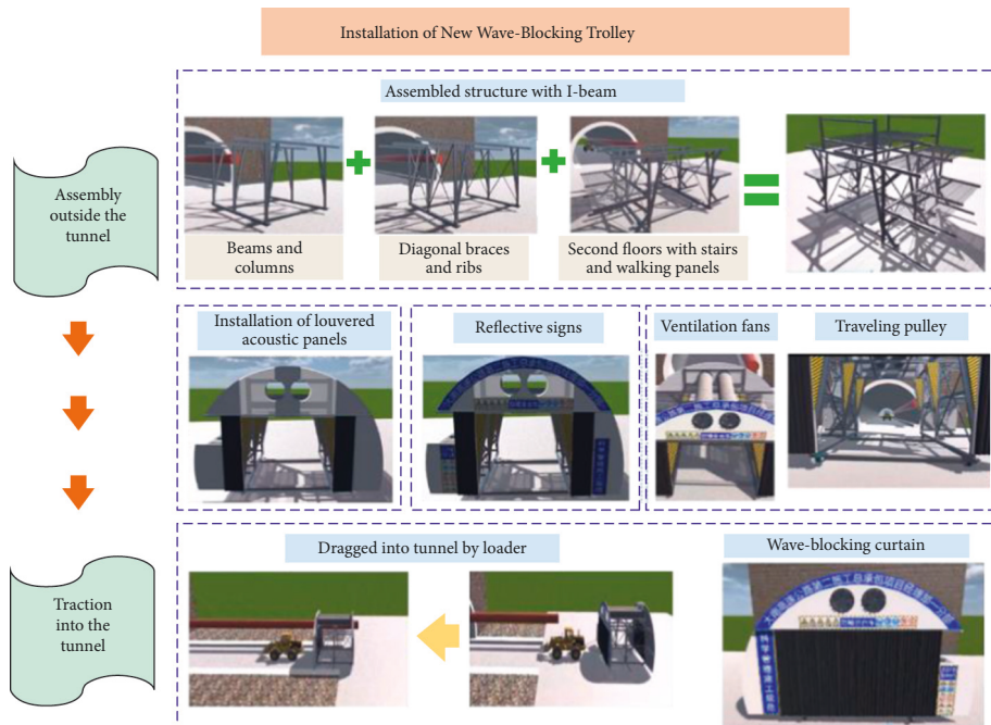
FIGURE 5: Installation of NWBT.
