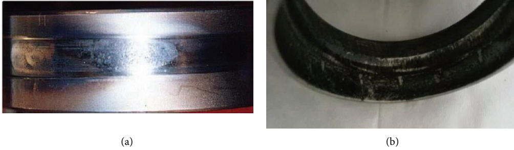
FIGURE 1: Bearing damage caused by thermal effect. (a) Bum of inner raceway. (b) Lubrication failure.
