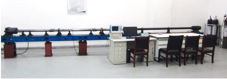
FIGURE 2: SHPB test apparatus.
