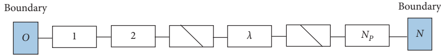
FIGURE 2: The monocoupled periodic structure of N_p cells with a free end (N) and a fixed end (O).
