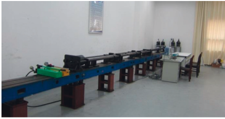
FIGURE 3: Split Hopkinson pressure bar test system.
