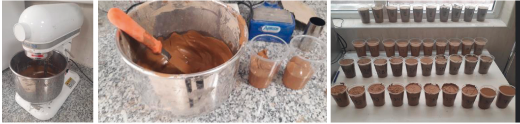
FIGURE 6: Mixing of stabilizing materials in research.
