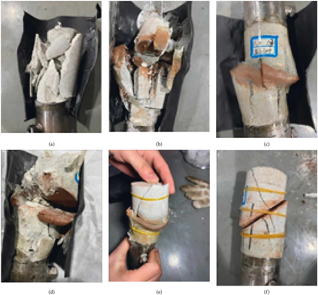
FIGURE 6: Fragmentation characteristics of mudstone specimens with different joint plane angles: (a) standard mudstone specimen, (b) joint plane angle of 15°, (c) joint plane angle of 20°, (d) joint plane angle of 25°, (e) joint plane angle of 35°, and (f) joint plane angle of 40°.
