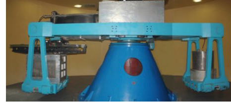
FIGURE 1: CKY-200 geotechnical centrifuge.
