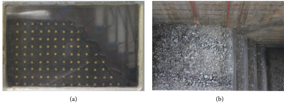
FIGURE 11: Photographs of RS4 embankment centrifuge model after test. (a) Side view. (b) Top view.
