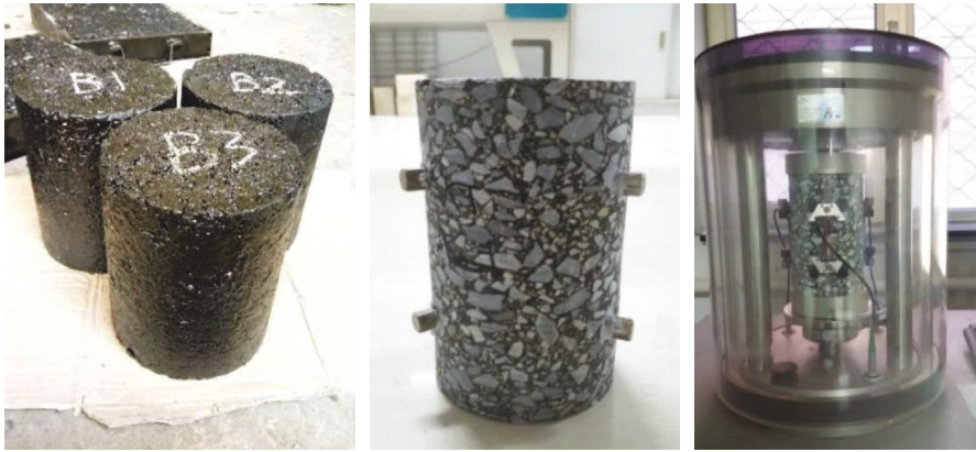
FIGURE 1: Uniaxial compressive strength test.
