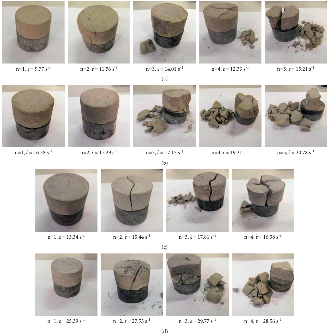
FIGURE 5: Combination of specimen failure pattern impact process. (a) I_p = 0.2 \text{ MPa} , DM-CTB 1:4 . (b) I_p = 0.24 \text{ MPa} , DM-CTB 1:4 . (c) I_p = 0.2 \text{ MPa} , DM-CTB 1:6 . (d) I_p = 0.24 \text{ MPa} , DM-CTB 1:6 .
