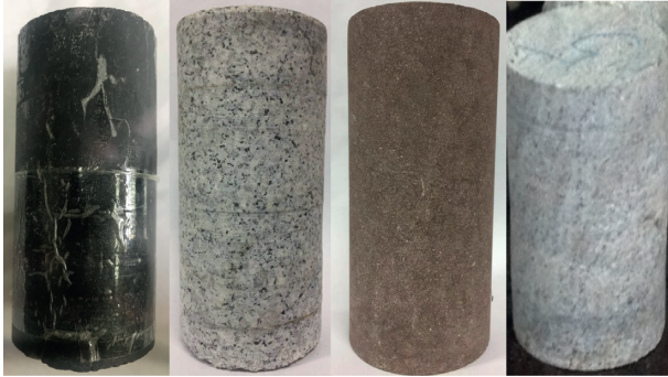
FIGURE 1: Rock types tested in the work (slate, granite, red sandstone, and limestone).
