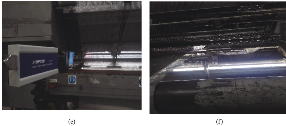
FIGURE 6: Vibration test positions. (a) Motor spindle. (b) Needles. (c) Hook bed. (d) Linkage. (e) Hook driven shaft. (f) Bottom pressing plate.
