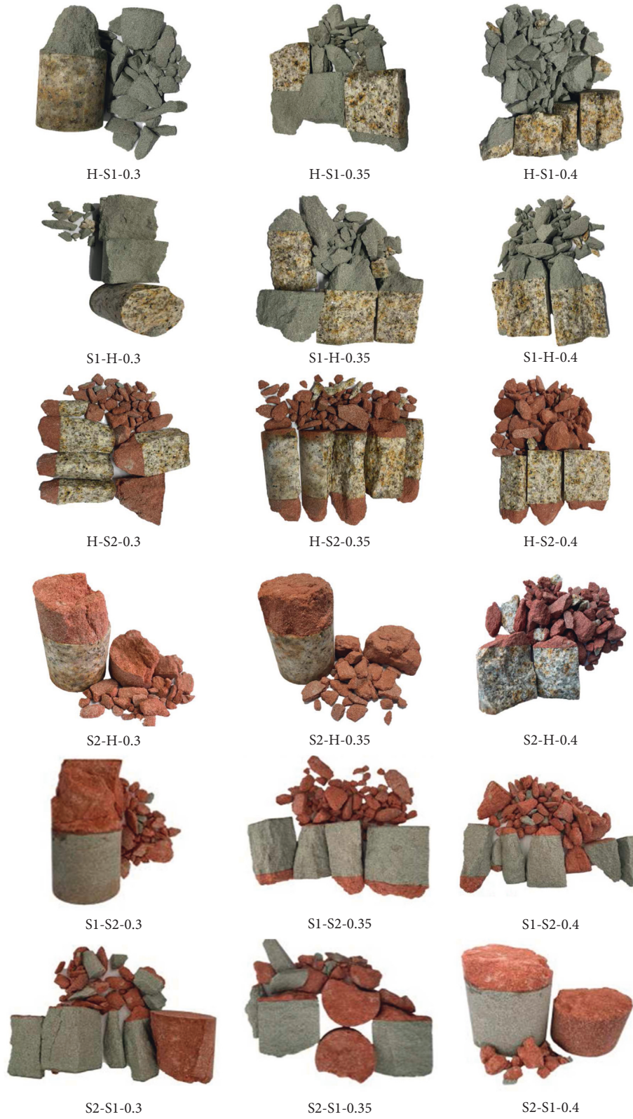
FIGURE 13: Failure photographs of composite samples after impact of dynamic loadings.
