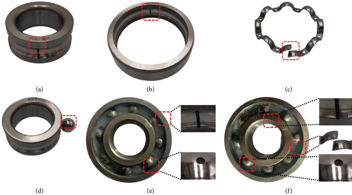
FIGURE 12: Different defect types in the experiment rig: (a) inner race (IR), (b) out race (OR), (c) cage, (d) ball, (e) out race and ball (OB), and (f) inner race, ball and cage (IBC).
