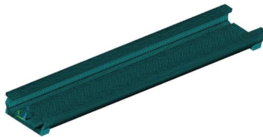
FIGURE 2: Finite element model of the U-shaped girder.
