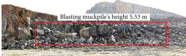
FIGURE 5: Blasting muck pile's height map.
