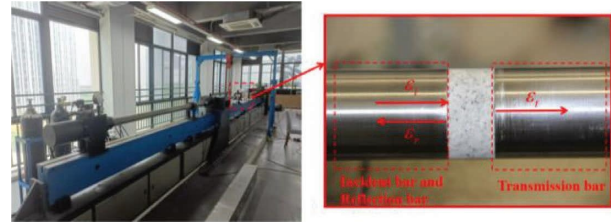
FIGURE 1: Split Hopkinson pressure bar test device.
