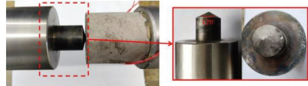
FIGURE 2: Dynamic point load test bar and sample installation.
