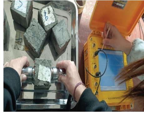
FIGURE 2: Filled body acoustic field test.
