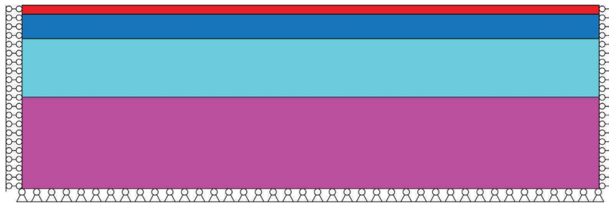
FIGURE 4: Boundary conditions of the simulation model.
