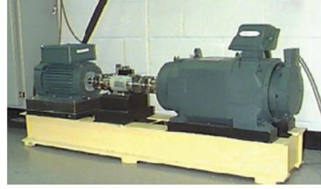
FIGURE 2: Rolling bearing test bench.
