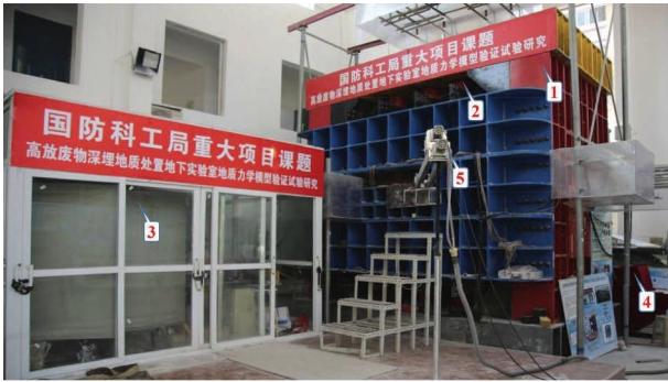
FIGURE 3: Three-dimensional geomechanical model test system: (1) reaction force device; (2) ground stress simulation system; (3) displacement monitoring system; (4) reaction force device; (5) micro-TBM excavation device.
