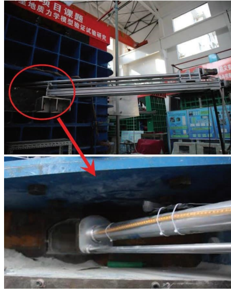
FIGURE 8: Photos of the micro-TBM excavation device.
