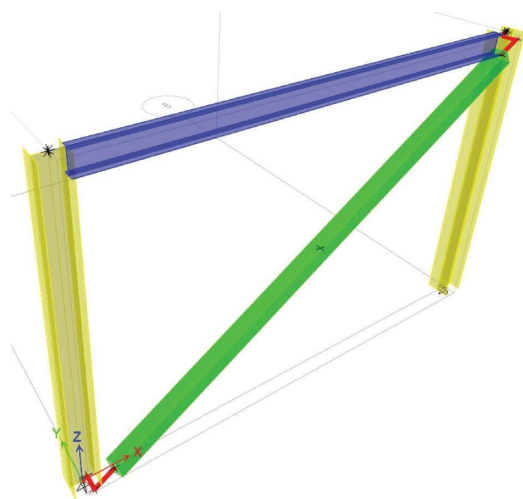
FIGURE 9: The frame with BIE element with e = 180 mm.
