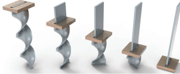
FIGURE 3: The ideal deformation process of the torsion plate.
