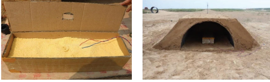
FIGURE 4: Explosive and placement.
