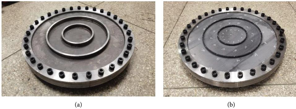
FIGURE 8: Stiffened circular sector plate under the fixed boundary condition. (a) Q235 steel. (b) Carbon fiber composite material.
