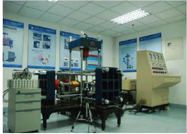
FIGURE 1: Deep rock burst process simulation test system.
