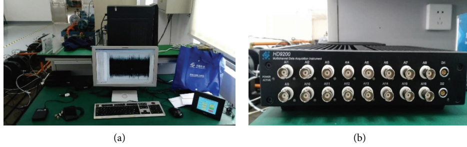
FIGURE 9: Operating platform and data acquisition system. (a) PC platform. (b) Data acquisition system.
