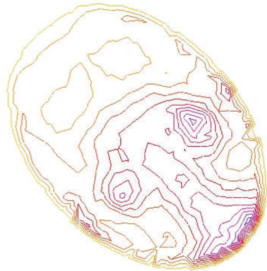
FIGURE 6: The kinetic energy value spatial distribution area in the objective runner.
