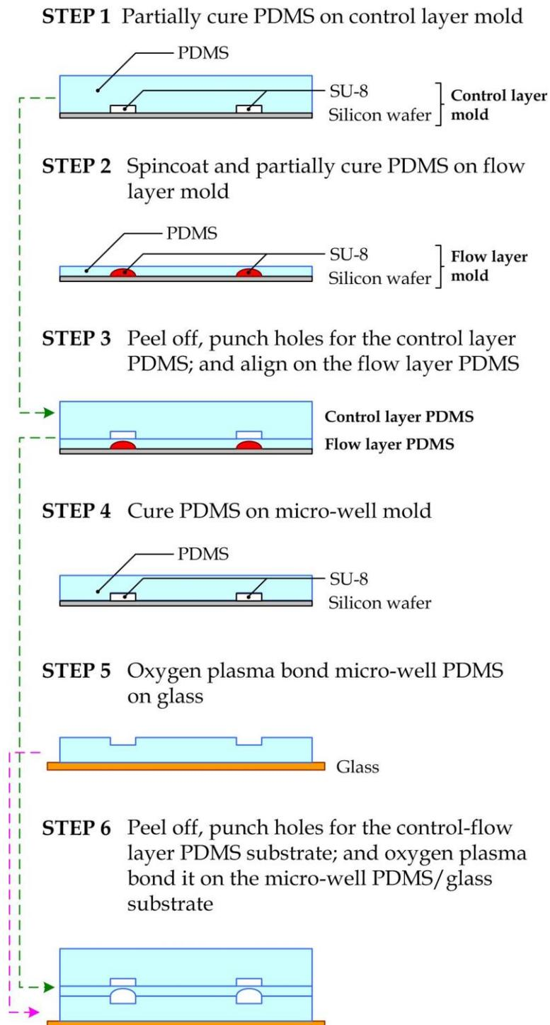
**Figure S3.** Illustration of the microfluidic device fabrication based on soft lithography.
